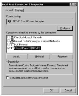
Figure 5-8. Adapter Properties for TCP/IP direct Connect
